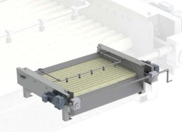
Waste is collected and can be removed underneath the machine. For spraying off sticky parts, the machine is provided with a spraying pipe over the rollers.
